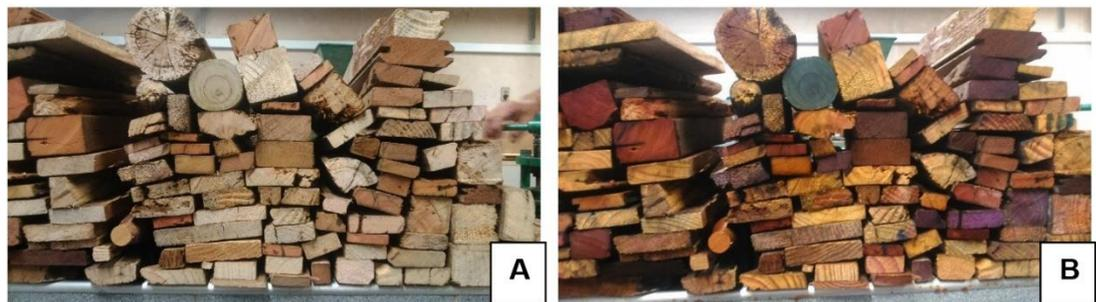
**Figure 3.** Samples submitted to a colorimetric test. (A) before the test and (B) after the test. The sample that presented a positive result to the colorimetric test was inserted to allow the comparative effect.
