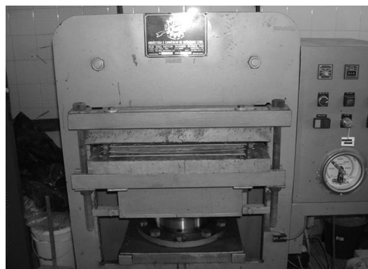
Figura 4 Prensa carregada com 3 painéis (1 Tratamento) (Loaded press with 3 panels (1 Treatment))
