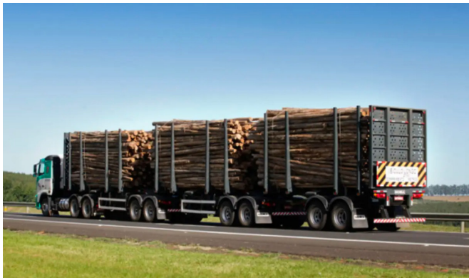
Figure 1. The most common tractor and trailer combination used in Brazilian pulp mills.
