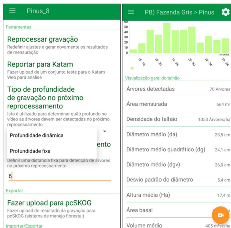
Figure 3 – Katam Forest app interface displaying the average results from one sampled line, processed with a fixed depth of 6 meters, along with the corresponding results for the entire plot
